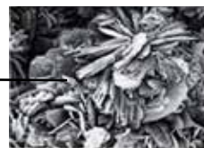
Accelerated osteointegration through full-surface, bioactive calcium phosphate coating (BONIT)
